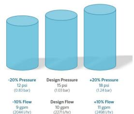
Figure 1. A system is designed to operate at 15 psi (1.03 bar). If this same system experiences a 20% pressure variation, that will result in a 10% flow variation. That small flow variation can negatively impact sprinkler performance and affect your yields.
