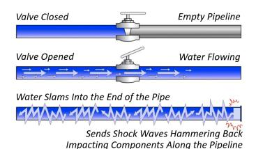
Figure 9. (Water hammer, 2018) illustration of what happens inside pipes including water hammer
