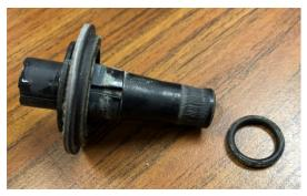
Figure 8. Scarred throttling stem from a worn pressure regulator.
