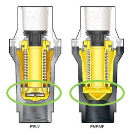
Figure 10. Comparing the seats of a limit valve versus a pressure regulator
