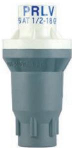
The Senninger PRLV (Pressure Regulating Limit Valve) is designed to be used in place of a standard water pressure regulator to limit static (no flow) water pressure when a shut-off valve is used downstream from the regulation point.
