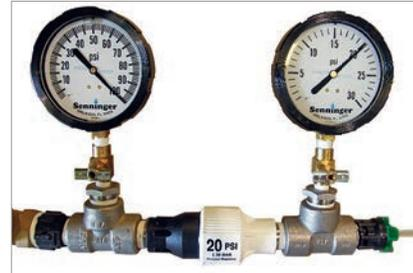
*If your irrigation dealer has a regulating testing device, you can also check the readings on a new pressure regulator that matches the model you are testing.*
