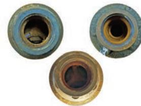
*Inlet and outlet of worn pressure regulators.*
