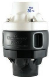
The Senninger PRXF-LV (Pressure Regulating Extended Flow Limit Valve) is designed to be used in place of a standard water pressure regulator to limit static (no flow) water pressure when a shut-off valve is used downstream from the regulation point.
