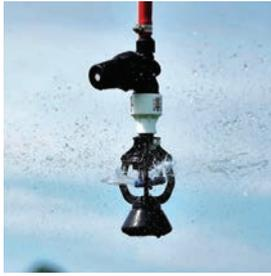
The Senninger® Filter Regulator helps prevent clogging of the small nozzles on the first few spans of a center pivot. This solution integrates filtration and pressure regulation in one product to provide installation convenience and help ensure optimal system performance.
