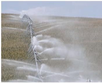
The Senninger® Pivot Master impact sprinklers distribute water in a low 6° trajectory and are designed to resist wind-drift. Their large diameter of throw means fewer sprinklers are needed.
