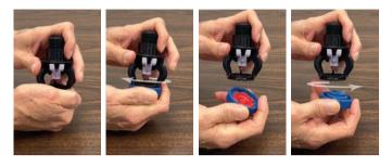
The LDN<sup>®</sup> offers chemigation pad inserts for corn or cotton. These are designed to produce an upward spray under the crop canopy to wash the underside of the leaves, where pests might hide. To change from irrigation to chemigation mode, simply twist and unlock the deflector pad. Flip it over and twist to lock it back in place. Any LDN Pad can be backed with a corn chemigation pad or a cotton chemigation pad insert.
