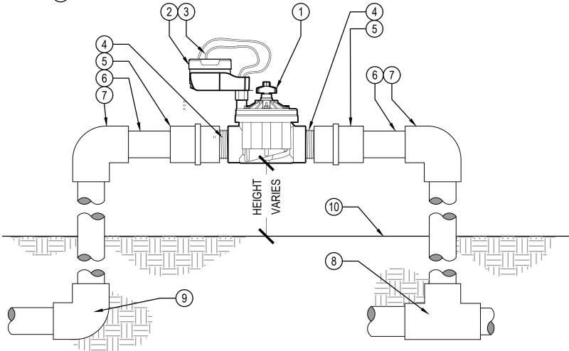
IN-LINE VALVE (ICV) WITH CONTROLLER (SENNODEBT)
