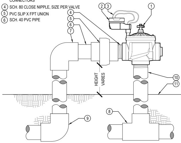
**ANGLE VALVE (ICV) WITH CONTROLLER (SENNODEBT) AND UNION**
