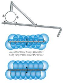
Truss Rod Hose Slings WITH Sling Finger Booms at the tower
