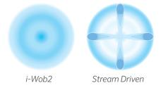
In this example, the i-Wob2 is instantaneously spreading the same amount of water over an area five times greater than the area covered by the spray nozzle.
