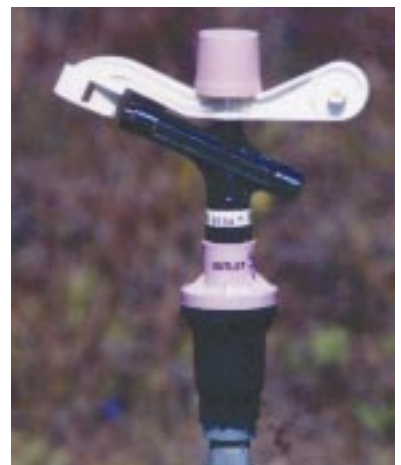
The sprinkler is a Senninger 4023 single nozzle F-luent-Master™, specially designed for effluent solutions. The assembly also includes a Senninger Medium Flow Pressure-Master Regulator® with a preset operating pressure of 50 psi.
